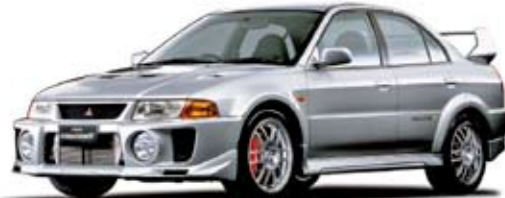
EVO V Launched in January 1998, the Evo V got an upgraded body kit, 17" rims, lighter pistons, plus a new ECU. The improved turbocharger pumped up 373Nm peak torque.
