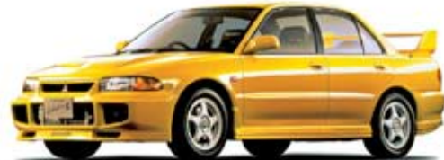
EVO III The Evo III arrived in January 1995, delivering an additional 10PS of peak power with an unaltered torque. It could do a top of 240km/h and 0-100km/h in 4.9 seconds.
