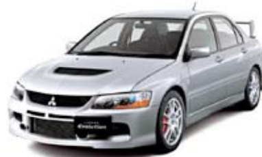
EVO IX The Evo IX came in 2005 with a 6-speed transmission variant and an increased peak torque of 407Nm.
