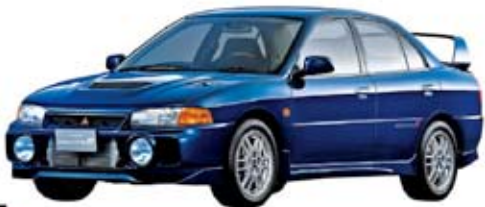
EVO IV A completely revamped Lancer arrived in 1996, in the form of Evo IV. The engine and transaxle rotated 180 degrees to eliminate torque steer. The car had a peak torque of 352Nm.
