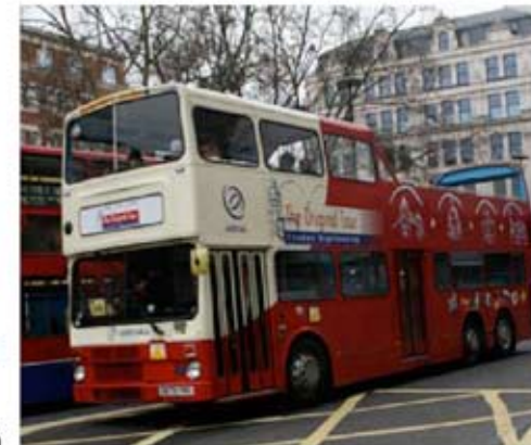
All London double deckers are now rear-engined and they come in either single rear axle or tandem rear wheel drive as on this tour bus.
