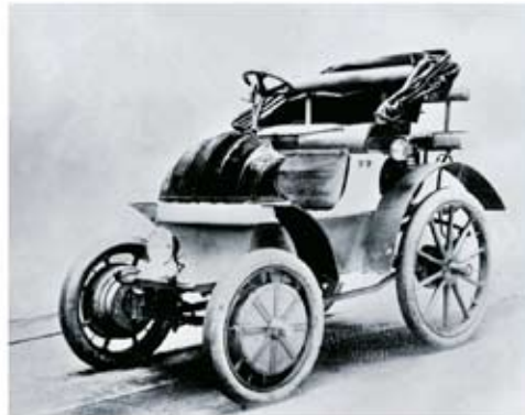
The very first Lohner-Porsche electric car powered by wheel hub motors was a sensation at the World Exhibition in Paris in 1900.
