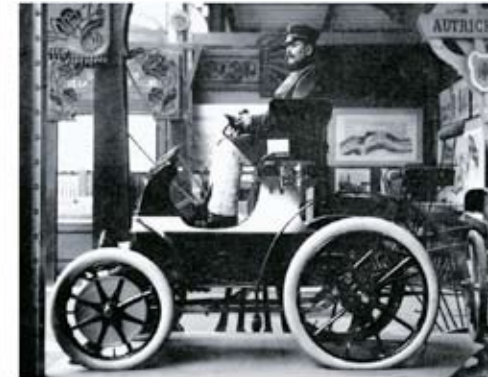
Evident in this pic are the large hub motors in the front wheels of this road-going Lohner, chauffeur waiting for his master to arrive.
