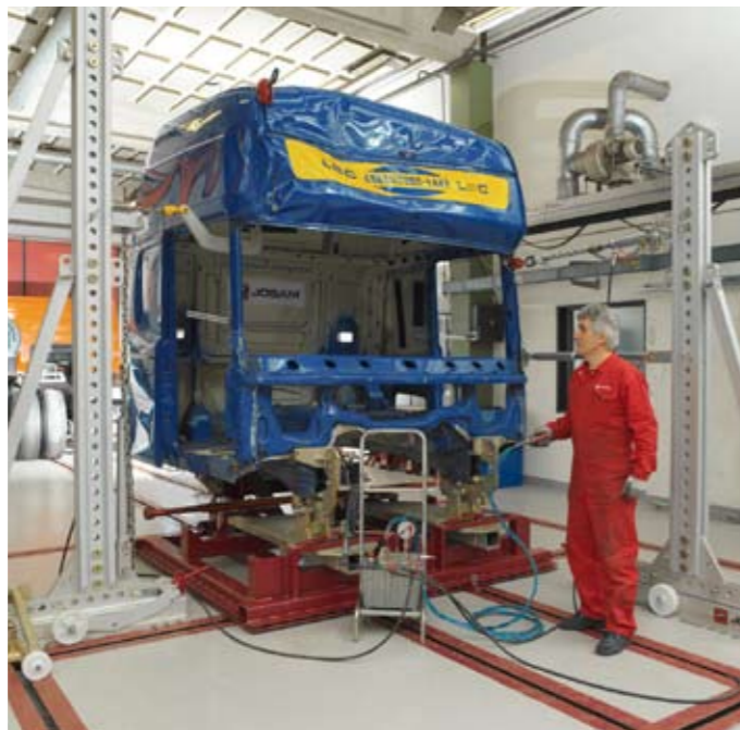
Josam cab tower anchored with I-beams as it straightens a cab.
