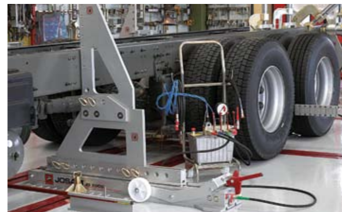
Josam frame straightening system aligns trucks and trailers up to 24 metres long and with an overall weight of 60 tonnes.
