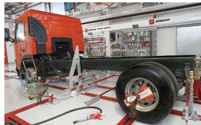
Josam frame straightening system aligns trucks and trailers up to 24 metres long and with an overall weight of 60 tonnes.
