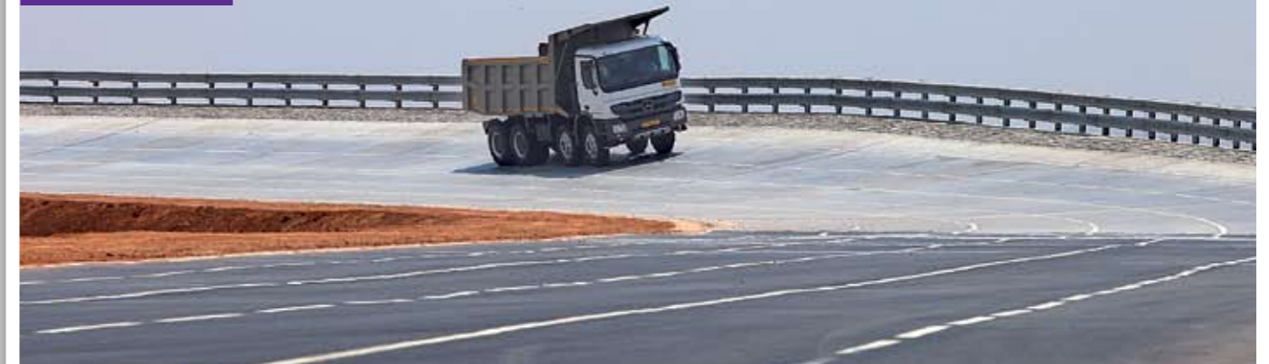
At Daimler Trucks' testing grounds near Chennai, vehicles can touch 90km/hour mark on the outer lane of the super-elevated section.
