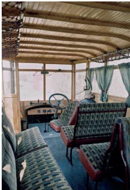
Functional aesthetics dominate with the traditional driver's position and the large flat windscreen giving ample forward vision. Note the simple mechanical driver-operated passenger door actuator on the dashboard.
