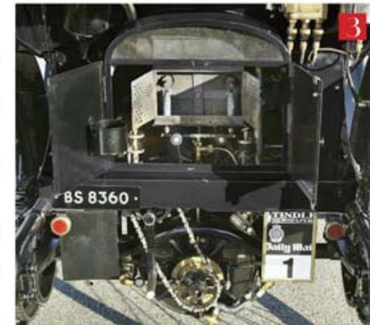
1 & 2 The immaculately maintained 1895 Vis-a-vis from the Louwman Collection was the No.1 car in the 2006 London to Brighton Veteran Car Run 3 Technology in 1895 allowed the 1282cc V-twin to make just about 3HP
